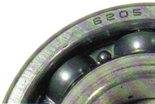
Bearing reference numbers allow you to order replacements cheaper from bearing suppliers, rather than paying the often hefty prices asked for 'official' spares
