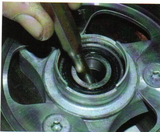
Using a drift to drive out a wheel bearing for inspection and possible replacement. Often driving a bearing out renders it unserviceable and replacement is the only option
